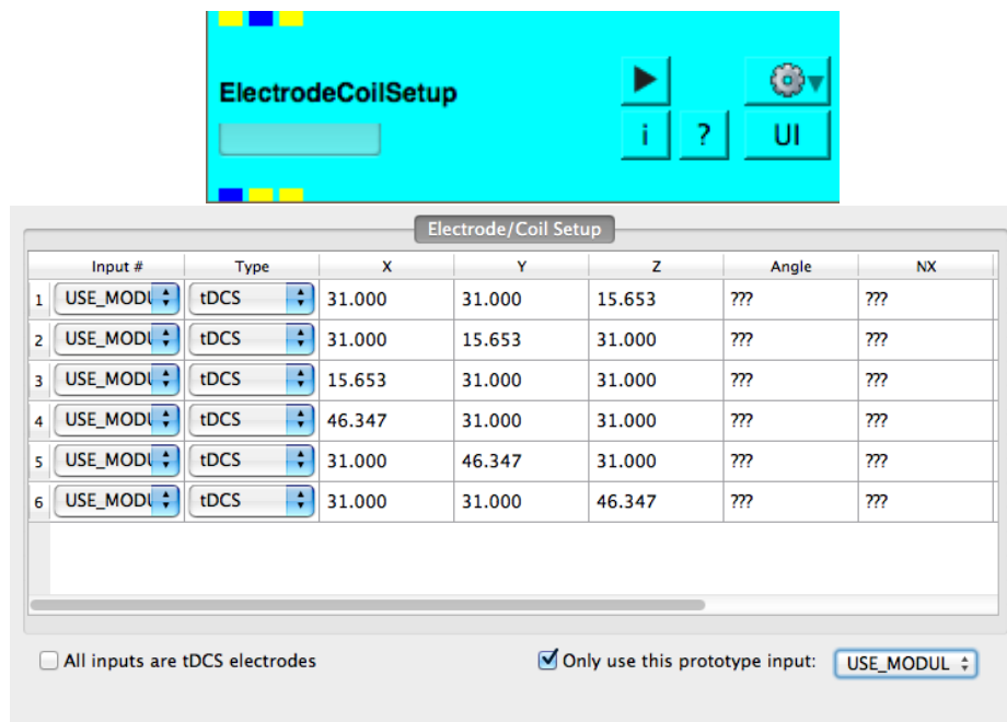
Figure 4.1. Electrode / coil setup module allows for electrode or magnetic coils properties to be manually inputted, such as the height, width, and length.
