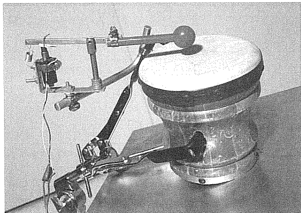
Figure 9. Sample motion module architecture: drumstick controlled by solenoid.
